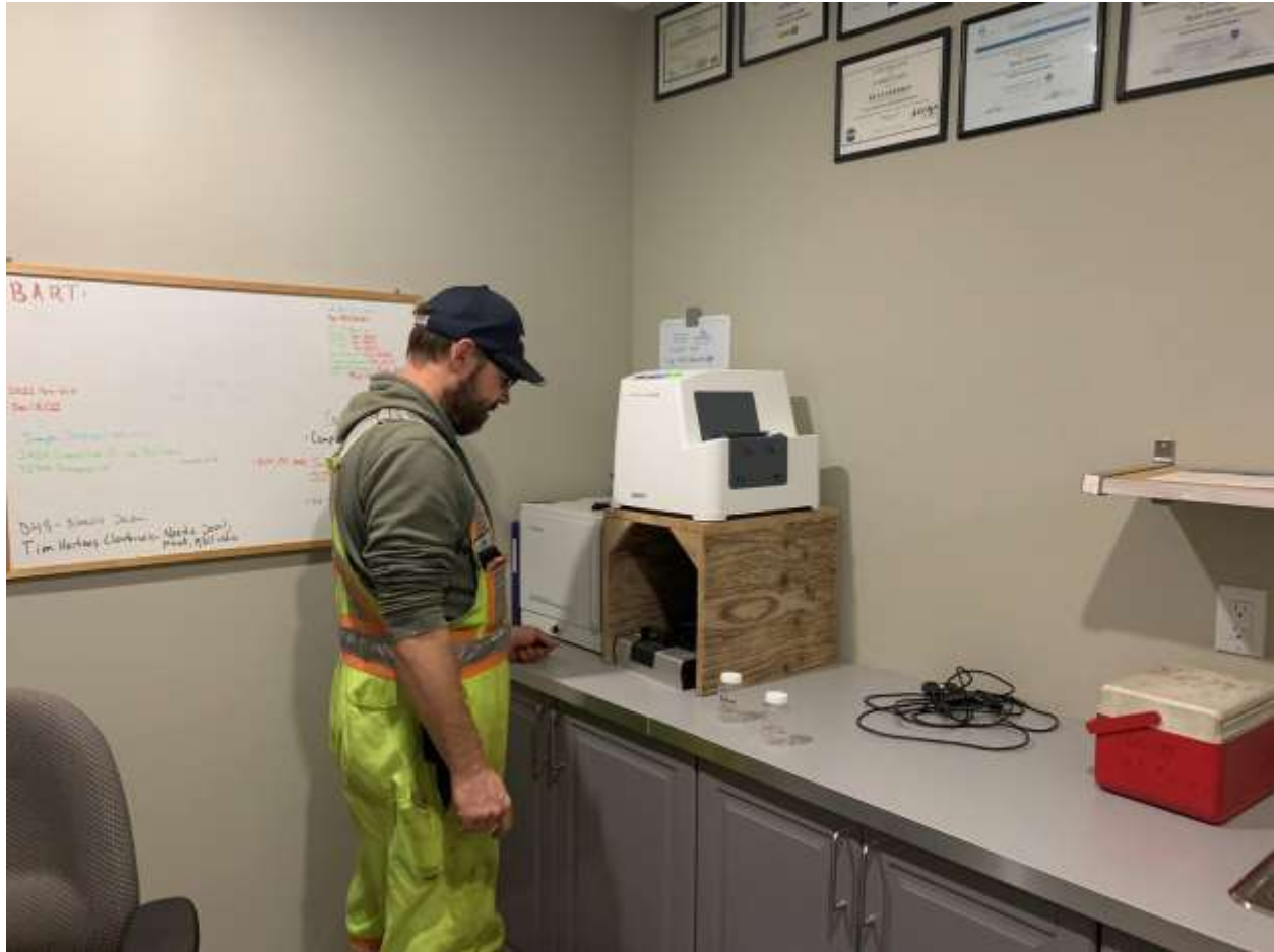
IMAGE | IN ADDITION TO WATER TESTING – IN HOUSE MICRO BIOLOGICAL ANALYSIS, WEEKLY COMPLETED BY THE WATER QUALITY TECHNICIAN, IN ADDITION TO WEEKLY WATER SAMPLES SUBMITTED TO THE BCCDC.
